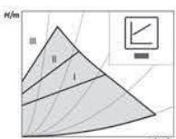
Recommended for two-pipe heating systems with radiators to reduce the flow noises at thermostatic valves.
